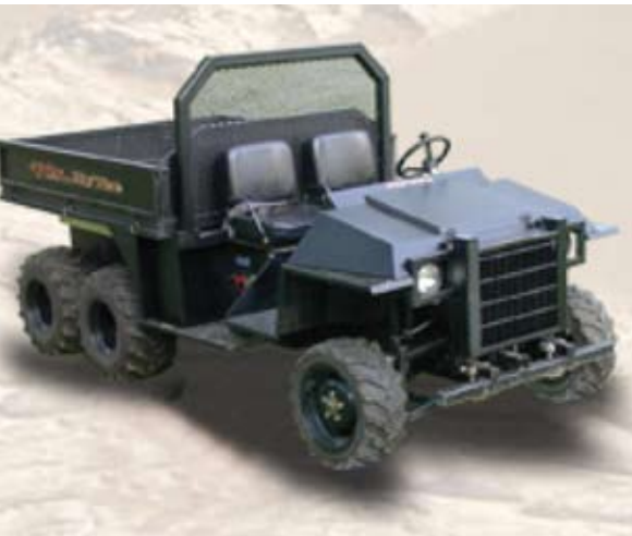
The basic version of the Hy Vee Ox may look like a souped-up golf cart, but its innovative hydrostatic transmission gives it impressive motive power, making it a valuable addition to military operations.
